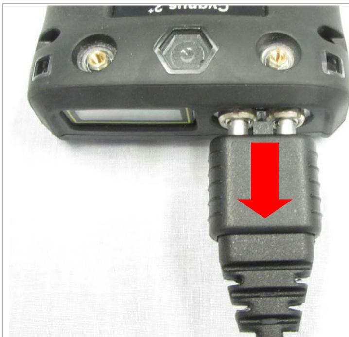
The connector is orientated with a 'pip' and can only be plugged in one-way around.
