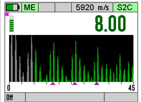
This A-Scan shows a Multiple-Echo measurement from a corroded steel sample.
