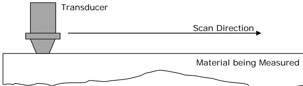
The results of the scan include a minimum thickness value. A cursor can also be positioned to pinpoint individual thickness measurements and log these to a data logger record if required. The B-Scan data is saved to a file on the SD card which can be transferred to CygLink for viewing and including in a Survey Report.
