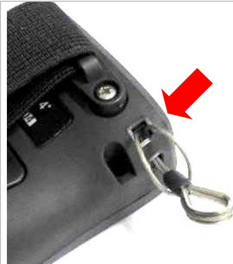
To fit the wire loop to the gauge body simply pass the loop through the hole in the gauge and back over the other end.
