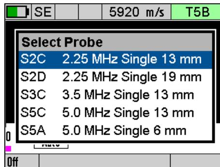
Manual Probe Selection – Single Element Probe Detected.
