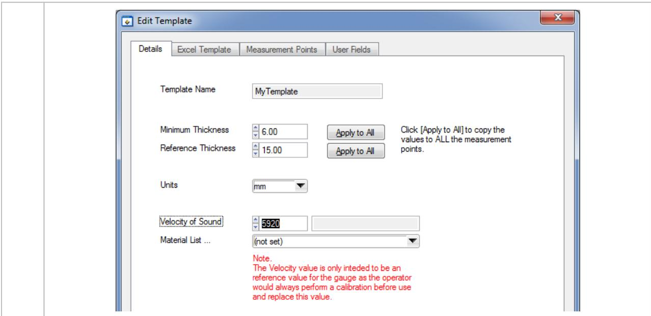
6. The **Measurement Points** tab lists each thickness measurement point in the order they will be taken. You can set the name, reference and minimum thicknesses and spreadsheet cell location.
