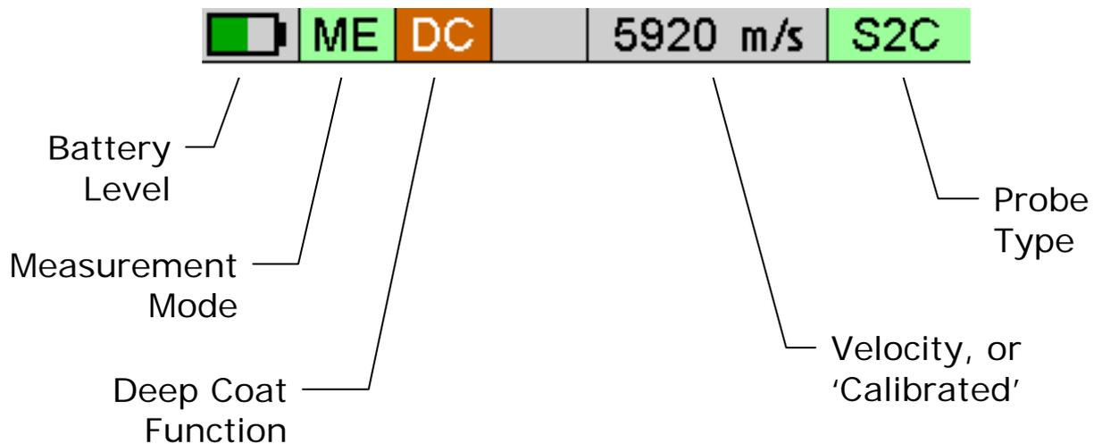
Probe Type; when the probe is connected the background colour is green, when disconnected it is grey.
