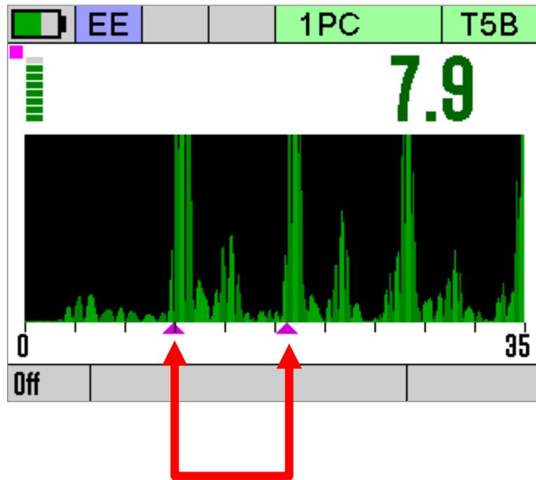
The gauge measures between these two echo signals to calculate the thickness. This is a good clear signal so the measurement is reliable.
