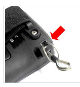
To fit the wire loop to the gauge body simply pass the loop through the hole in the gauge and back over the other end.
