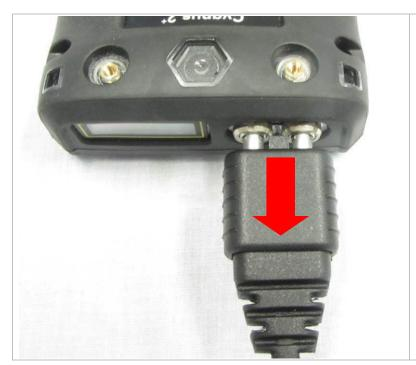
The connector is orientated with a 'pip' and can only be plugged in one-way around.
