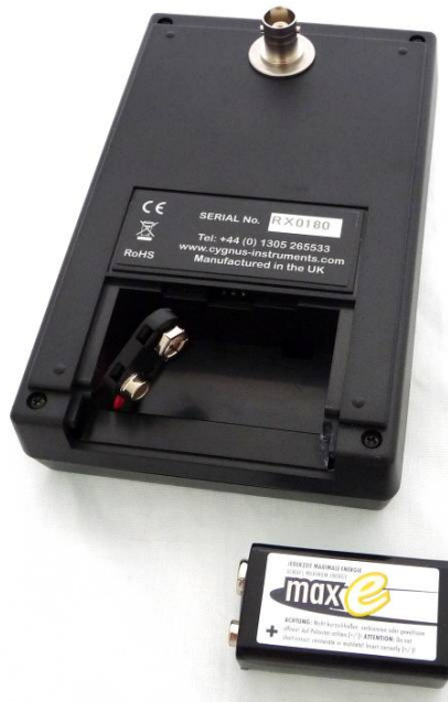
Fig 4.3 Receiver Battery Location
