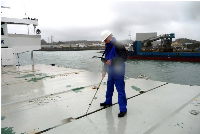
Fig 7.6. Scanning a Hatch Cover Joint.
