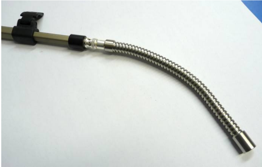
Fig 5.2 Inspection Microphone Connected to the Telescopic Extension
