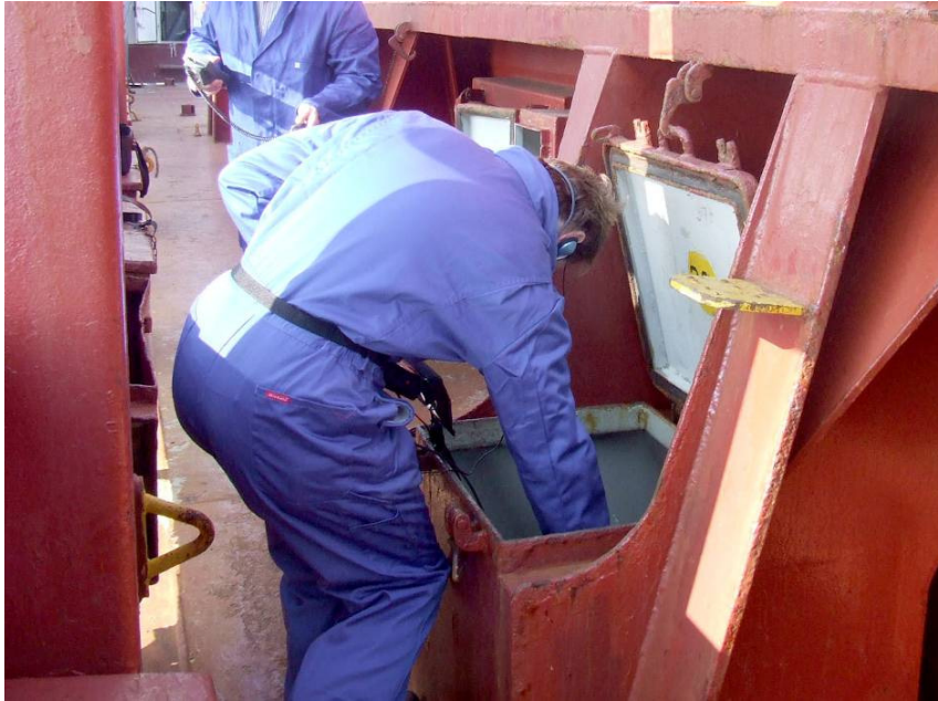
Fig 7.5 Setting an Open Hatch Value using an Access Hatch
