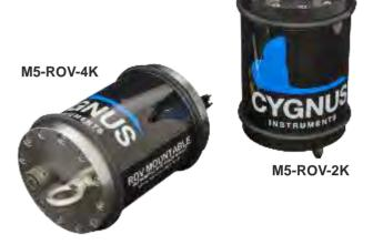
Specifically designed for underwater remotely operated vehicles, Cygnus offer two dedicated ROV mountable thickness gauges, M5-ROV-2K (depth rated 2,000 m) and M5-ROV-4K (depth rated 4,000 m). These gauges are versatile and designed to measure metal thickness through coatings in the harshest operating conditions.
