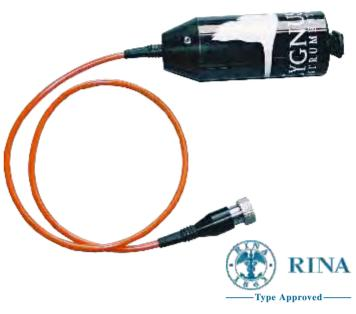
The Cygnus Mini ROV Mountable thickness gauge has been specially designed to be mounted onto small observation ROVs with or without a manipulator facility. Built in conjunction with VideoRay, this mountable subsea thickness gauge will allow the operator to carry out an ultrasonic thickness measurement in areas that have previously been infeasible using larger ROVs or divers. This Multiple-Echo thickness gauge measures metal thickness and corrosion without removing protective coatings.
