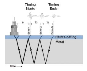
With Multiple-Echo, readings are taken by measuring the time delay between any three consecutive backwall echos. The time of T1 (coating thickness) is ignored. The times of T2 and T3 are equal to the time that it takes to travel through the metal. Only by looking at three echoes can the measurements be automatically verified (where T2 = T3).
