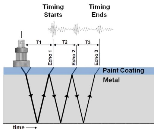
With Multiple-Echo, readings are taken by measuring the time delay between any three consecutive backwall echos. The time of T1 (coating thickness) is ignored. The times of T2 and T3 are equal to the time that it takes to travel through the metal. Only by looking at three echos can the measurements be automatically verified (where T2 = T3).
