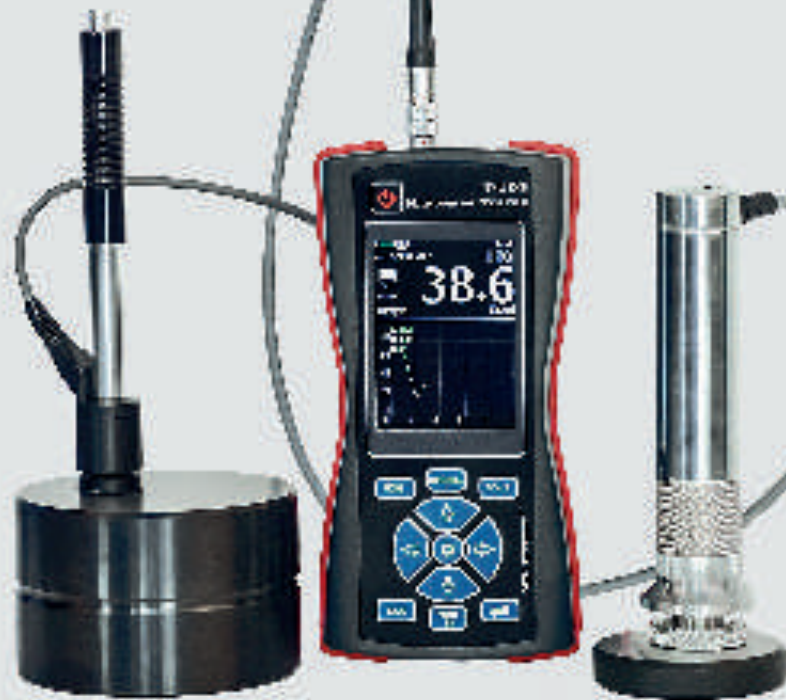
Leeb Probe ASTM A956
