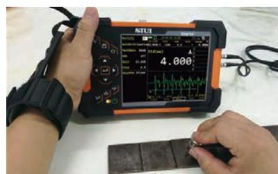
Thickness measurement on step block
