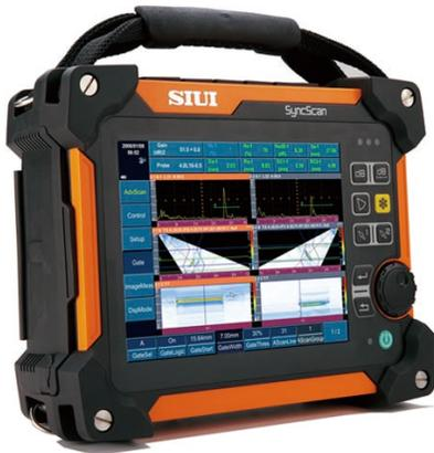
Latest ultrasonic flaw detector from SIUI, SyncScan incorporates the latest advancements in high-performance Phased Array and TOFD detection into one compact and durable unit. SyncScan can be upgraded with Phased Array, TOFD and thickness measurement to satisfy various inspection requirements.
