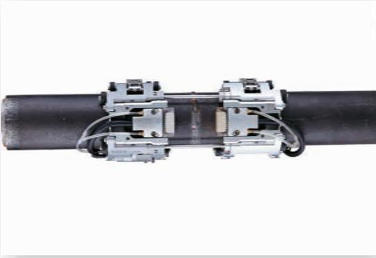
The PA bracelet crawler LPS-01 and LPS-02 are compatible with PA ultrasonic flaw detector, which is used to perform circumferential weld inspection on small diameter pipes.
